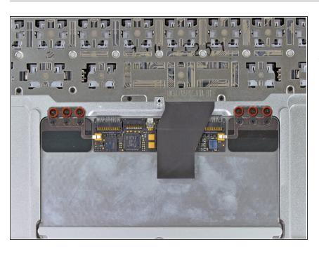
Remove the six 1.5 mm Phillips #00 screws that secure the trackpad assembly to the upper case.
