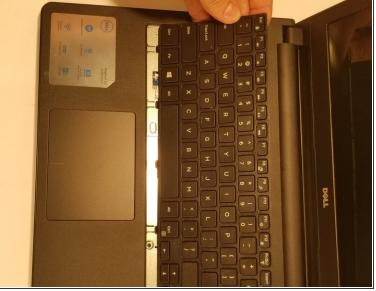
Lift the keyboard off of the computer. \*Be careful not to tear the ribbon that attaches the back of the keyboard to the computer when lifting it.\*
