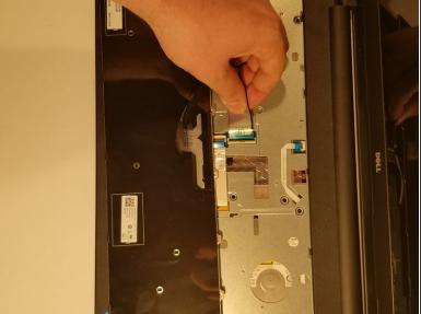
Flip the black securing bar near the base of the ribbon with a spudger to release the ribbon from the computer.
