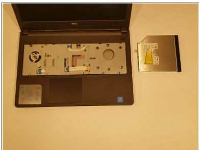
After all 3 screws are removed take a spudger and pry the CD-Drive out of the computer.
