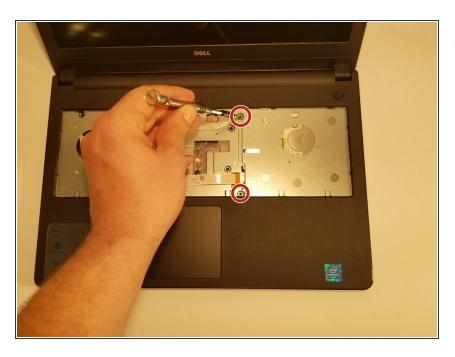
Next using the J0 bit tipped screwdriver unscrew the 2 remaining screws shown in the picture.
