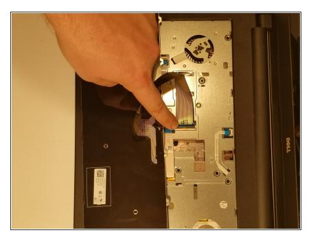
Flip the keyboard over onto the palm-rest assembly.
