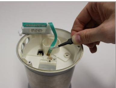
Pull out the green ribbon cable through the rubber cover.
