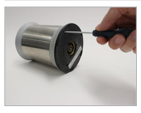
Remove the 12mm Torx screws (x3) from the bottom of the foamer using a Torx TR10 screwdriver.
