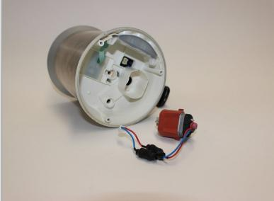
Remove the electromotor by hand.
