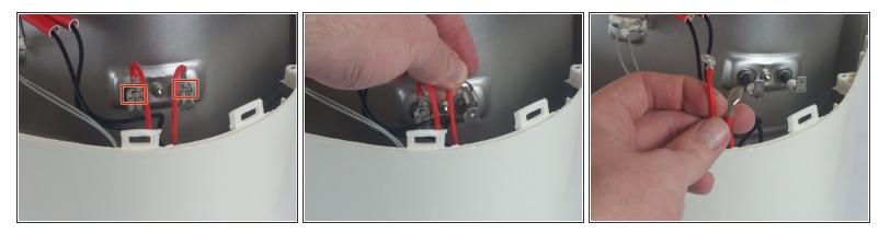
Disconnect the red wires from the inner liner.
