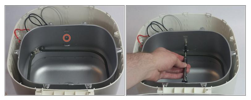
• Remove the single 11mm Phillips #1 screw thats holding and inner lining in place.
