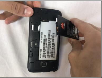
Use the flat end of a spudger, or fingernail, to lift up the battery and pull out.
