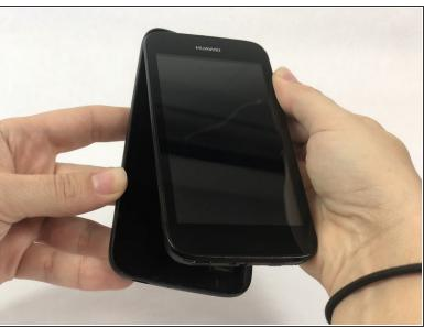
Wedge your thumb nail, or the flat end of a spudger, into the bottom left corner and pry off.
