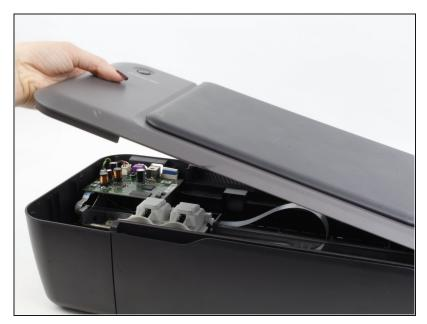
With the front of the printer facing you, lift and raise the left side of the panel (like opening a book in reverse) until it disconnects from the clip on the right side of the panel.
