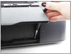
• In the front of the printer, open the tray where the paper comes out and remove the two 13 mm screws located under the top of the printer.
