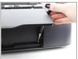
• In the front of the printer, open the tray where the paper comes out and remove the two 13 mm screws located under the top of the printer.
