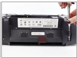
Remove the two 13 mm screws located on the back of the printer using a screwdriver with the T10 torx bit (star-shaped).
