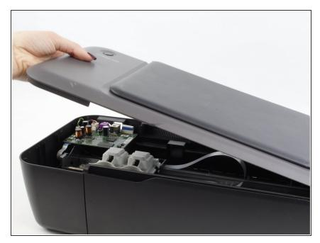
With the front of the printer facing you, lift and raise the left side of the panel (like opening a book in reverse) until it disconnects from the clip on the right side of the panel.
