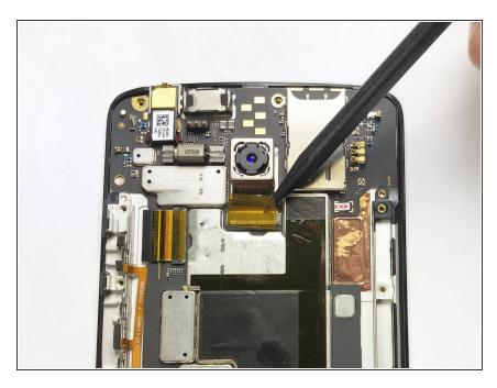
• Peel up orange adhesive that covers the ZIF connector.
