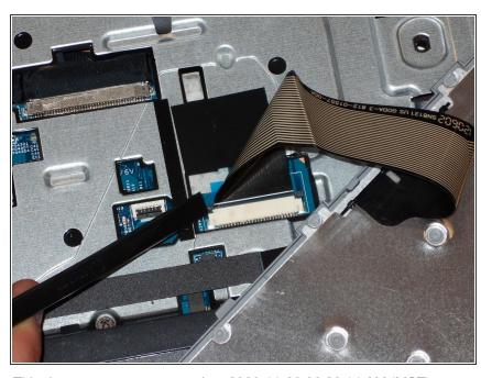
Use the spudger and slide the grey tabs on either side of the keyboard wires away from the white plastic.
