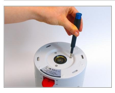
We start off with unscrewing the three screws from the bottom of the water kettle. Two of the three screws can be unscrewed with a Philips Ph 1.8 screwdriver. The other screw can be unscrewed with a spanner screwdriver.
