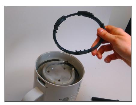
Here we end this part of the disassembly and go back to the main base of the kettle. From the bottom of the kettle, you see a black plastic ring. This can be removed by undoing the snap fits. This can be done easily by hand.
