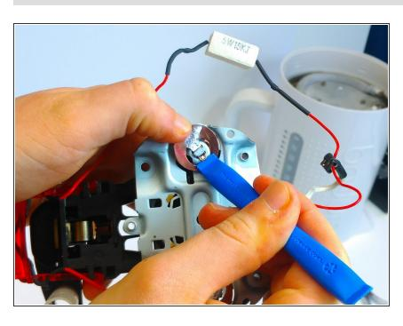
To continue, we focus on the black plastic parts that we just removed from the water kettle. On this are two metal rings located, these can be slipped out with the help of a levering tool. With the two rings, two little grey pins will come out.
