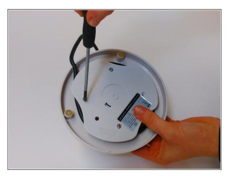
The base can be disassembled by unscrewing the four screws with a PH1 for three of them, and slightly less high PH1 with the other one.
