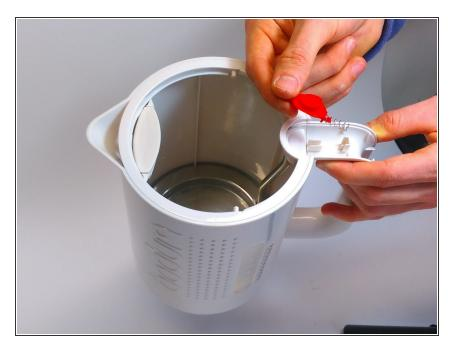
Then, you can remove the switch by just picking it up from the kettle.
