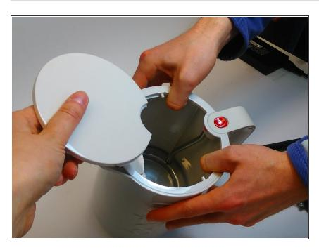
After removing the ring, flip the kettle and remove the lid by pulling the kettle a little bit to transform the circle,. You might need another pair of hands for this step.
