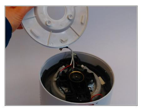
After unscrewing the screws, you can detach the bottom of the water kettle.
