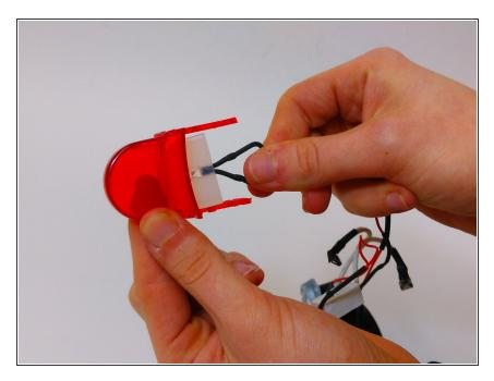
Next, you can remove the red casing from the light. This might take some power, so hold on to the light so you don't break the wire.
