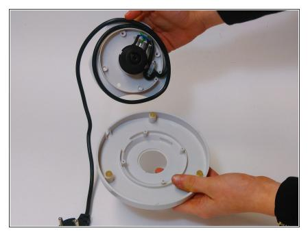
You can now remove the two parts to unveal the electronic part in the base.
