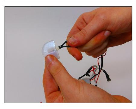
After removing the casing, you can remove the rubber filling in the same careful way. You now have access to the LED.
