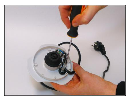
You can remove the electronic part by unscrewing the two screws with a PH1 screwdriver.
