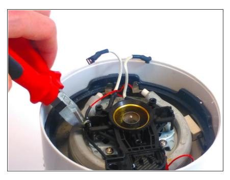
The next step is to cut the small zip tie, this can be done easily with a wire cutter.
