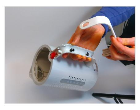
After this, you can remove the grip by sliding the snap fingers at the top, located at the switch, out. This can easily be done by holding the grip with your hand, and sliding the grip with your thumb.
