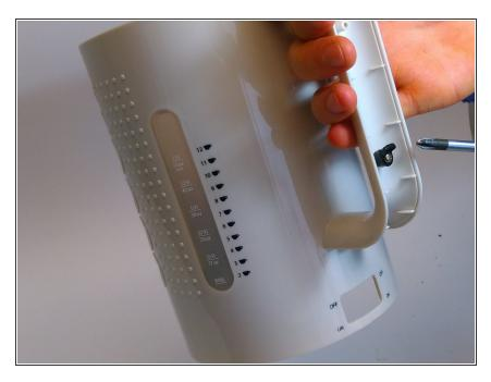
The screws with the black plastic that became visible with the removal of the grip can be unscrewed with a PH1 screwdriver.
