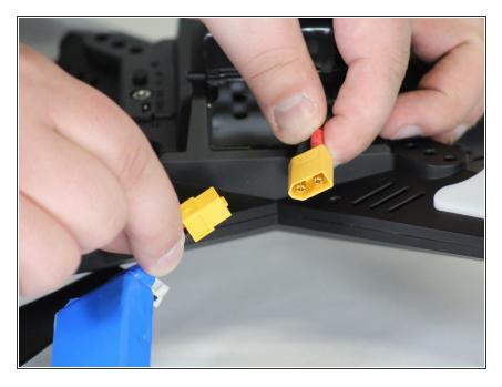
• Disconnect the two ends of the wires by lightly pulling them apart.
