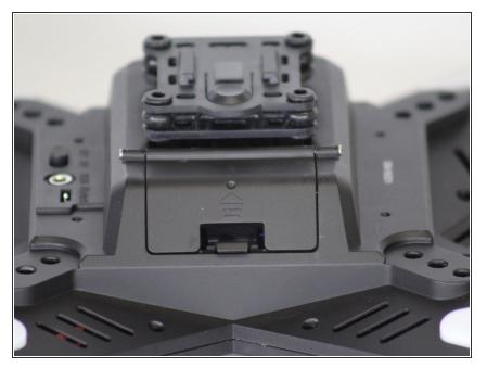
• Locate the door to the battery compartment on the underside of the drone.
