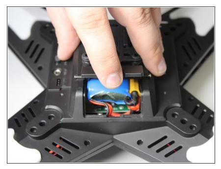
• Open the door to the battery compartment by pressing in the clip on the door and carefully lifting until the door is fully open.
