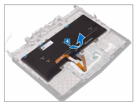
Lift the keyboard at an angle and remove it from the tabs on the palmrest assembly.
