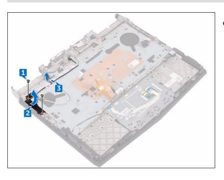
Lift the power-button board, along with its cable, off the palm-rest assembly.
