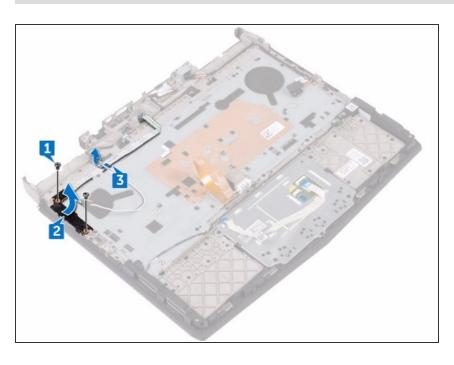
Align the screw holes on the powerbutton board with the screw holes on the palm-rest assembly.
