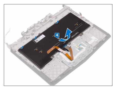
Align the tabs on the palm-rest assembly to the slots on the keyboard bracket and snap into place.
