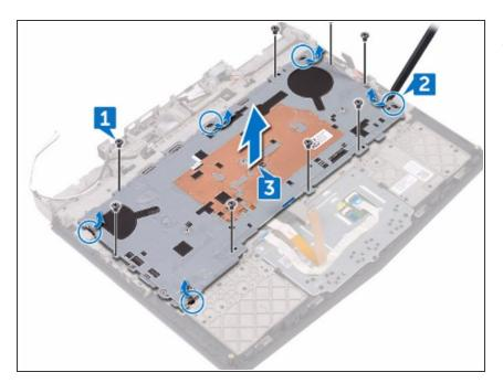
Replace the eight screws (M2x3) that secure the keyboard bracket to the palm-rest assembly.
