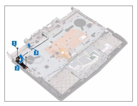
Adhere the power-button board cable to the palm-rest assembly.
