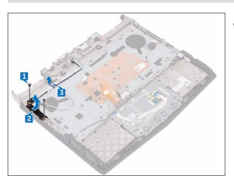
Using the alignment posts, place the NEW power-button board on the palm-rest assembly.
