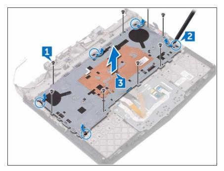
Using a plastic scribe, pry the keyboard bracket off the palm-rest assembly.
