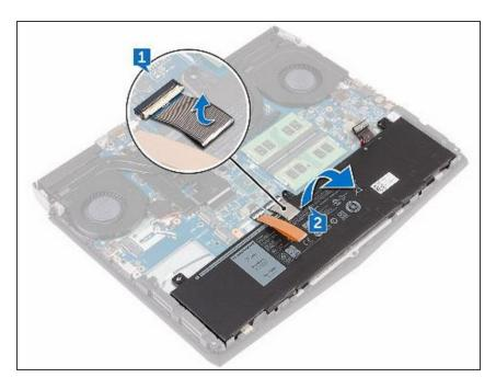
Lift the battery off the palm-rest assembly.
