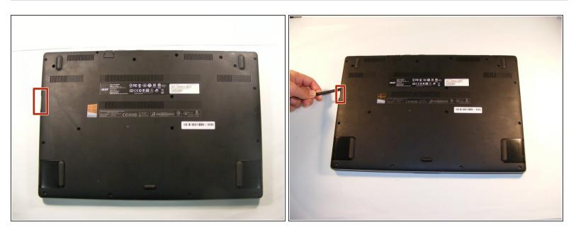
Use the spudger to slowly work your way around the perimeter starting at the marked location to pop the bottom cover off.
