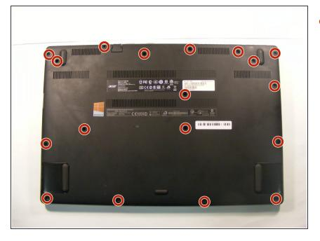
Remove all 18 marked screws (2.12 mm) using a Phillips #1 Screwdriver.
