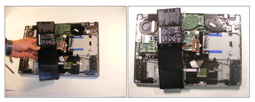
• Unplug the marked plug from the motherboard and this will complete the removal of the battery.
