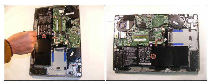
• Remove the 1 marked screw (3.3 mm) holding the battery in place using a Phillips #1 Screwdriver.
