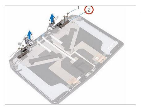
Lift the display hinges off the display back-cover.
