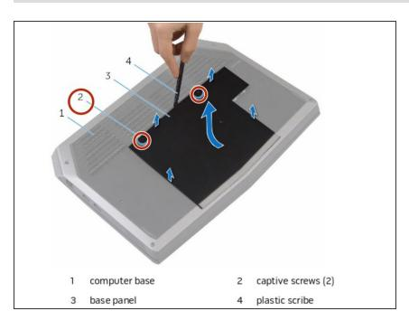
Loosen the captive screws that secure the base panel to the computer base.
