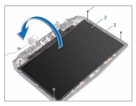
Connect the **NEW** display cable to the display panel and press down on the connector latch to secure the cable.
