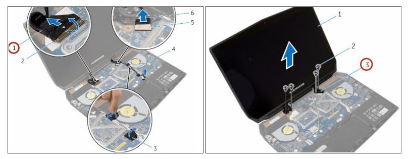
Remove the display cable from the routing guides on the display hinges.
