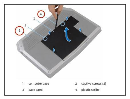
Using a plastic scribe, gently release the tabs that secure the base panel to the computer base.
