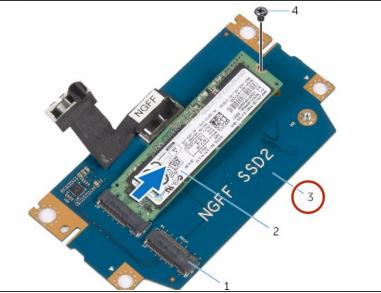
Replace the screw that secures the solid-state drive to the solid-state drive assembly.
