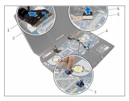
Adhere the adhesive tapes that secure the antenna cables to the system board.
