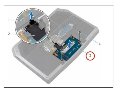
Lift the solid-state drive assembly off the computer base.
