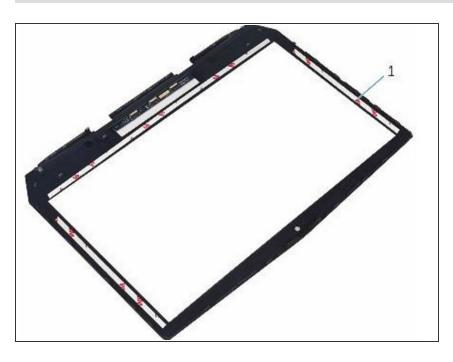
Align the display bezel with the display back-cover and gently snap the display bezel into place.
