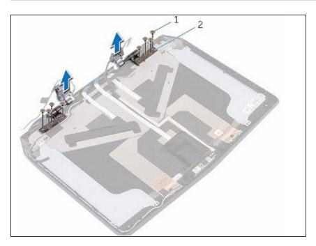
Replace the screws that secure the display hinges to the display backcover.
