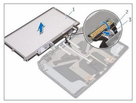
Connect the **NEW** display cable to the display panel and press down on the connector latch to secure the cable.
