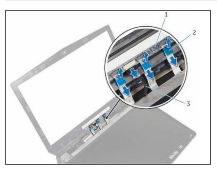
Slide the display-board cables to their respective connectors on the logo board and press down the latches to secure the cables.
