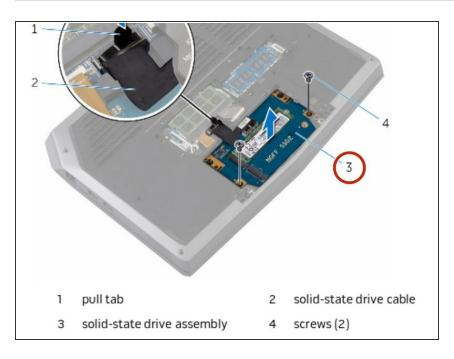
Align the screw holes on the solidstate drive bracket with the screw holes on the solid-state drive assembly.
