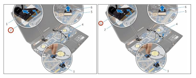
Lift the connector latch and disconnect the display cable from the system board.
