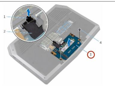
Remove the screws that secure the solid-state drive assembly to the computer base.
