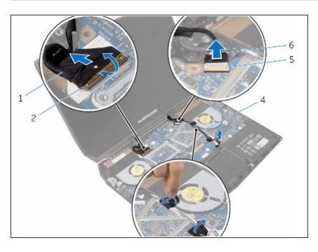
Slide the display cable into the connector on the system board and press down the latch to secure the cable.
