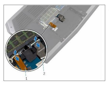
Lift the latches and disconnect the keyboard and keyboard-backlight cables from the system board.
