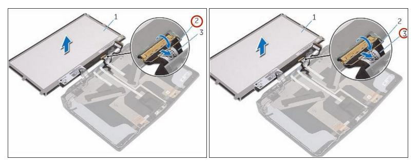
Lift the connector latch and disconnect the display cable from the display panel.
