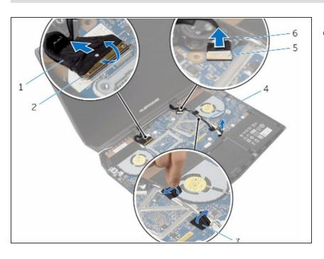
Route the logo-board cable through the routing guides on the display hinge and connect the logo-board cable to the system board.
