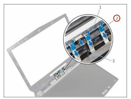
Lift the connector latches and disconnect the display-board cables from the logo board.
