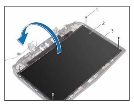
Align the screw holes on the display panel with the screw holes on the display back-cover.
