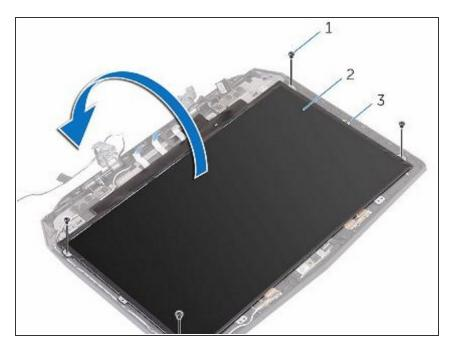
Replace the screws that secure the display panel to the display backcover.
