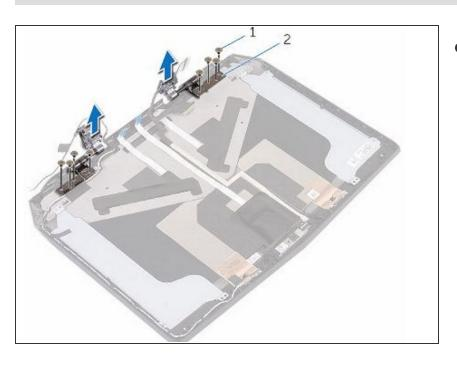
Align the screw holes on the NEW display hinges with the screw holes on the display back-cover.
