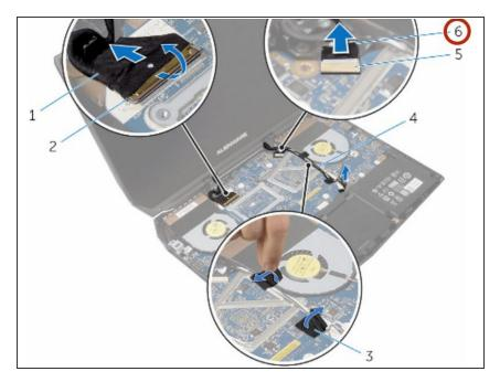
Disconnect the logo-board cable from the system board and remove it from the routing guides on the display hinges.
