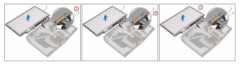
Lift the connector latch and disconnect the display cable from the display panel.
