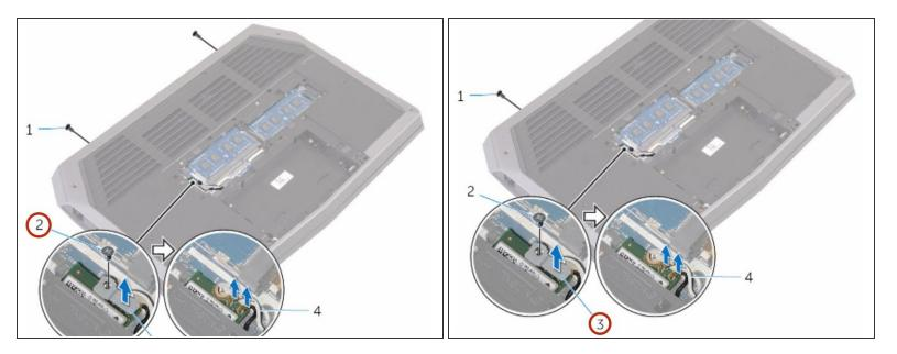
Remove the screw that secures the wireless-card bracket to the wireless card.
