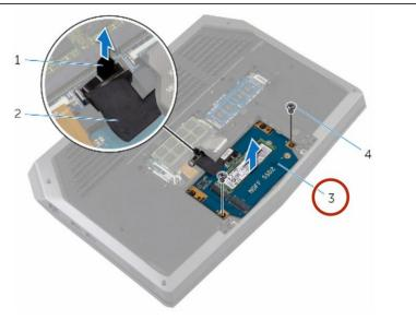
Align the screw holes on the solid-state drive assembly with the screw holes on the computer base.
