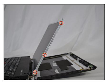
Remove the plastic covering and six 1.3mm Phillips #00 screws from both sides of the display.
