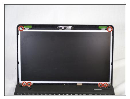
Remove the six 1.3mm Phillips #00 screws from around the display.
