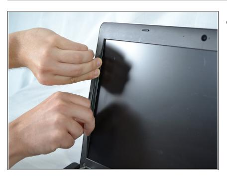
Slide your finger underneath the plastic and pry gently to release the clips around the display bezel.
