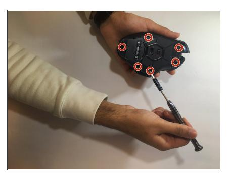
Use a Phillips #00 screwdriver to unscrew all 6 screws (3x5mm) from under the mouse feet.
