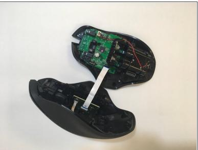
• Lift the top of the mouse from the base of the mouse (separate the mouse in half) to expose the internal hardware.
