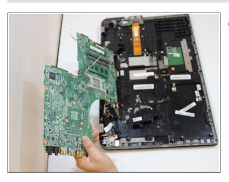
Disconnect all wires from the motherboard and replace motherboard.
