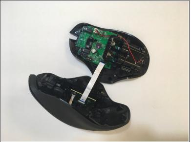
• Lift the top of the mouse from the base of the mouse (separate mouse in half) to expose the internal hardware.
