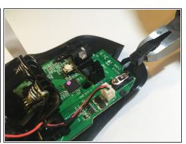
Use pliers to grip and remove the black covers over the button — the black cover and the button, a small white plastic piece, should come off).
