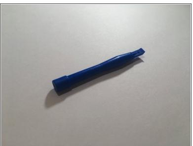
Use a blue spudger to open the bottom battery port.
