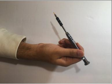
• Use a #00 screwdriver (3x5mm) to unscrew all 6 screws from under the mouse feet.
