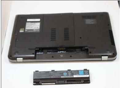
Lift the battery upwards and remove it from the device.
