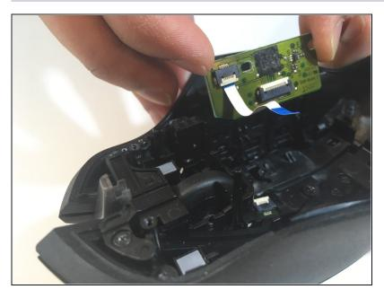
Use a black spudger and your fingers to loosen and remove the side motherboard.
