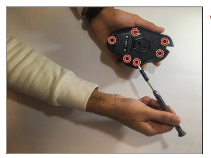
Use a Phillips #00 screwdriver to unscrew all 6 screws (3x5mm) from underneath the mice feet.
