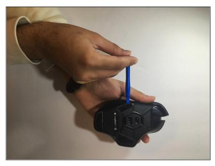
Use a blue spudger to pry all 4 mice feet from the bottom of the mouse.
