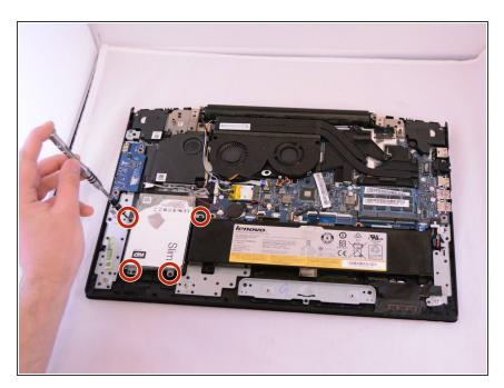
Use the Phillips #0 screwdriver to unscrew the four screws.
