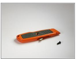
The case screw can easily be removed by using a Stanley #2 screwdriver or any other #2 screwdriver.
