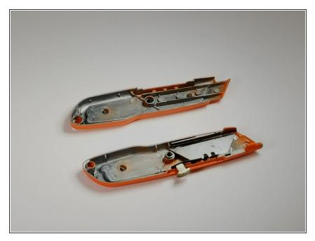
Separate casing by simply pulling apart both halves.
