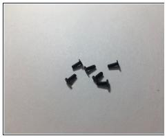
• Use a Phillips #00 screwdriver to unscrew all 6 screws (3x5mm) from under the mouse feet.
