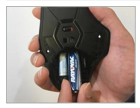
Remove the two AA batteries from the device.
