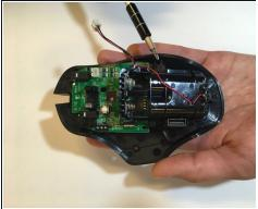
Use a Phillips #00 screwdriver to unscrew all 5 screws (3x5mm) from the battery pack and motherboard.
