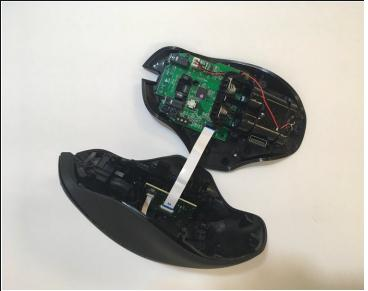
• Lift the top of the mouse from the base of the mouse (separate mouse in half) to expose the mouse's internal hardware.
