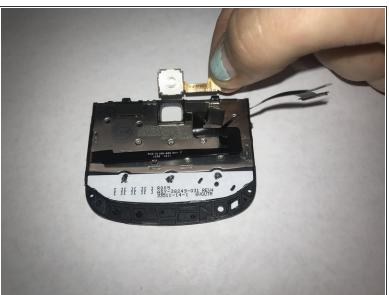
• The trackpad is attached via ribbon cable. Pull this cable up in order to release the trackpad.
