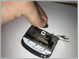
• Push into the trackpad. This will release the trackpad supporting piece.
