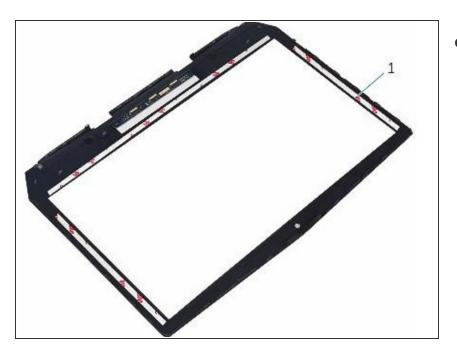
Align the display bezel with the display back-cover and gently snap the display bezel into place.
