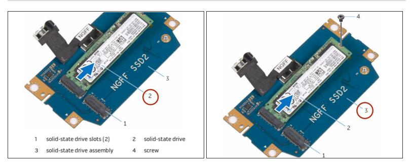
• Replace the screw that secures the solid-state drive to the solid-state drive assembly.
