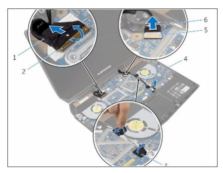
Route the logo-board cable through the routing guides on the display hinge and connect the logo-board cable to the system board.
