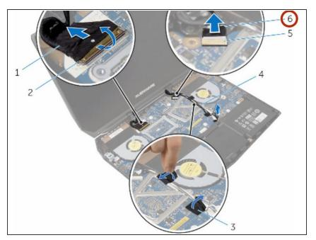
Disconnect the logo-board cable from the system board and remove it from the routing guides on the display hinges.
