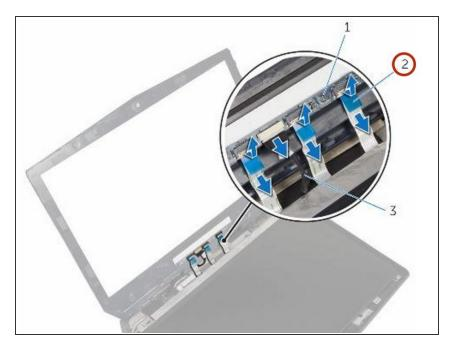
Lift the connector latches and disconnect the display-board cables from the logo board.
