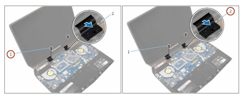
• Remove the screws that secure the hinge caps to the display hinges.
