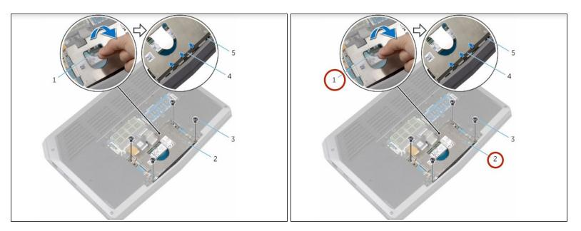
Using the pull tab, pivot the solid-state drive bracket and peel off the bracket from the tabs on the computer base.
