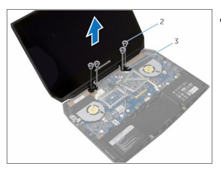
Align the screw holes on the hinge caps with the screw holes on the display hinges.
