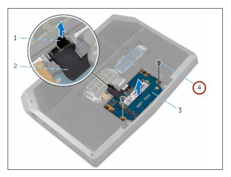
Remove the screw that secures the solid-state drive to the solid-state drive assembly.
