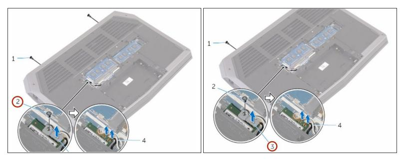
• Remove the screw that secures the wireless-card bracket to the wireless card.
