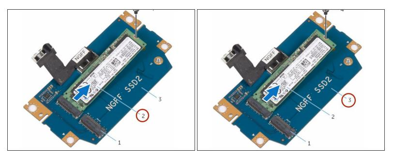
• Replace the screws that secure the solid-state drive bracket to the solid-state drive assembly.
