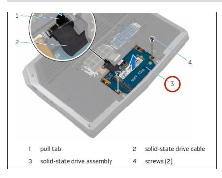
Align the screw holes on the solidstate drive bracket with the screw holes on the solid-state drive assembly.
