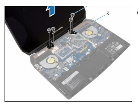
Align the screw holes on the display hinges with the screw holes on the computer base.
