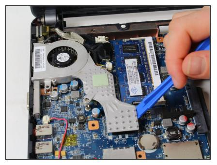
• Using the plastic opening tool, pry up the unscrewed fan.
