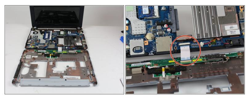
• Open the top carefully without disconnecting the two parts.
