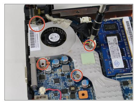
• Use a Philips #0 screwdriver to unscrew the 4 heatsink screws.
