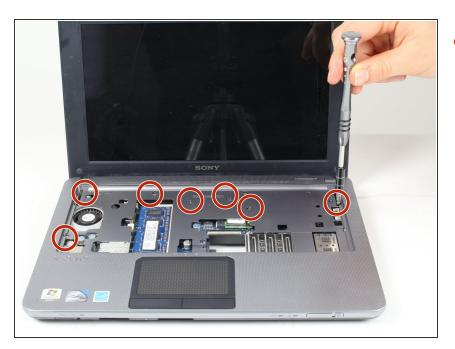
Use a Philips #0 screwdriver to remove the 7 top case screws.
