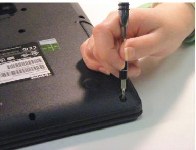
Using the Phillips #1 screwdriver, remove the eleven 2.5mm screws.
