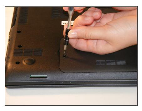
Remove the one 2.5mm Phillips #1 middle plate screw.
