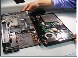
Using the plastic opening tool, remove the outer panel and set to the side.
