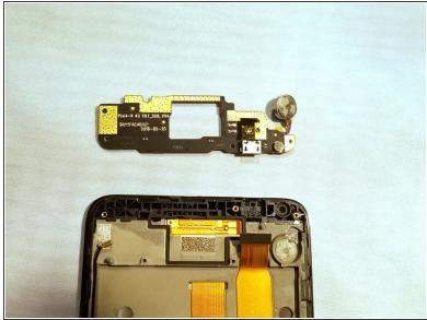
Using the black spudger, pry off the board the USB charging port is attached to.
