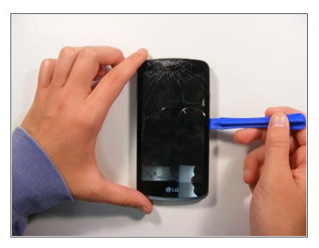
Insert the plastic opening tool into the groove between the screen and the rest of the device. Work your way around the perimeter by sliding the opening tool around the edge, loosening the screen.
