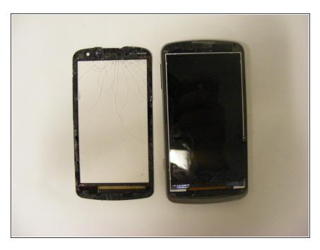
Once the screen is loosened, fully remove it from the device by peeling it away from the base of the phone.
