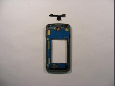
• On the front side of the phone, push down on the top plastic shield to loosen it, and remove the shield using the plastic opening tool .
