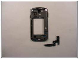
On the back side of the phone, loosen the bottom shield using the plastic opening tool, and remove it from the device.
