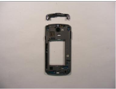
On the back side of the phone, remove the upper shield using the plastic opening tool.
