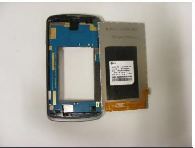
Insert plastic opening tool into groove between display and body of the phone. Work your way
