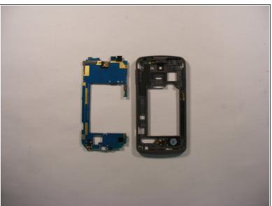
Using your fingers, grab onto the blue motherboard and safely remove the loosened motherboard from the device.
