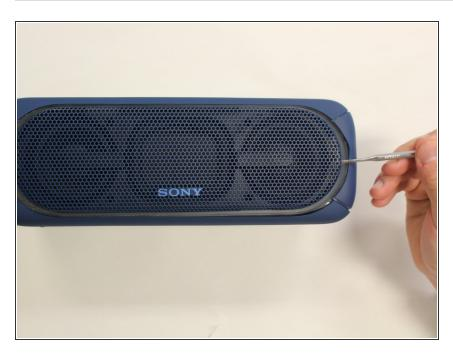
Remove the speaker case from the outer casing by prying it from the base of the speaker using a metal spudger.
