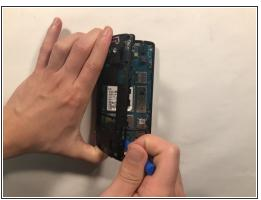
Once the back is removed you will have access to the 8 screws that need to be unscrewed with the Phillips #0 screwdriver. Once all screws are free use the opening tool to pry the back frame of the phone apart.
