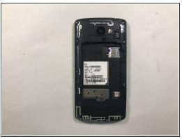
Pry the back of the phone open in the incision area at the bottom of the phone with your opening tool in an upward direction to retrieve access to the battery.
