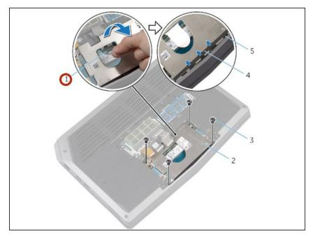
Using the pull tab, pivot the solidstate drive bracket and peel off the bracket from the tabs on the computer base.
