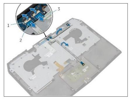
Slide the touchpad cable and the status-light cable into their respective connectors on the powerbutton board and press down the latches to secure the cables.
