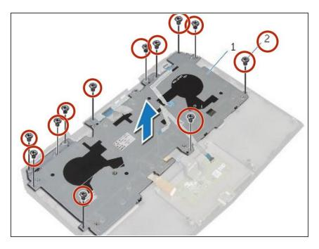
Remove the screws that secure the keyboard to the palm-rest assembly.
