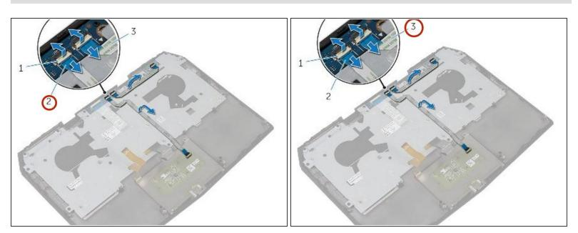
Adhere the touchpad cable and status-light cable to the keyboard bracket.
