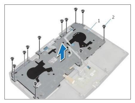
Replace the screws that secure the keyboard bracket to the palm-rest assembly.
