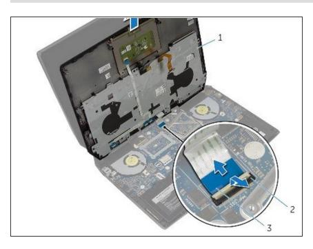
Connect the power-button board cable to the system board.
