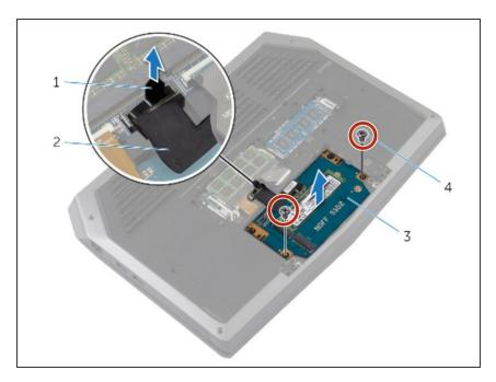
Replace the screw that secures the solid-state drive assembly with the screw holes on the computer base.
