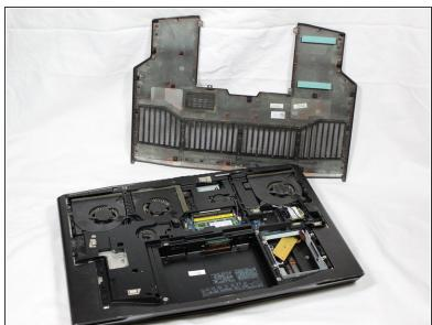
Use the plastic pryer tool to lift the bottom cover off.
