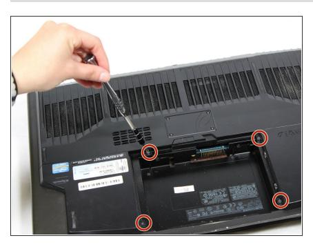
Unscrew four screws with a J000 screwdriver.
