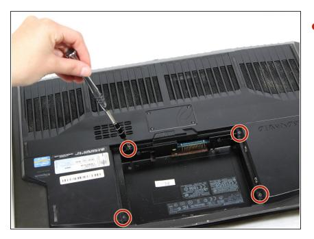
Unscrew the four indicated screws with a J000 screwdriver.
