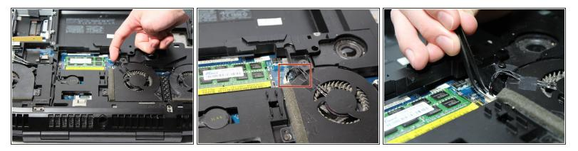
The fan will be connected to the motherboard by a cable. Use plastic tweezers to gently unplug this connection.
