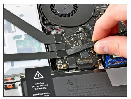
• Use the flat end of a spudger to pry the hard drive cable connector up from its socket on the logic board.
