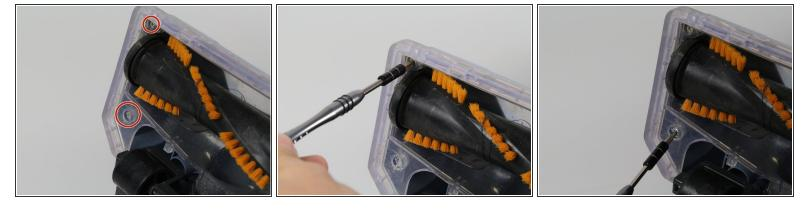
Remove the two screws on the left side of the brush.
