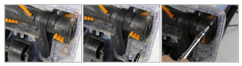
Use a Phillips #1 screwdriver to remove the two screws on the right side of the brush.
