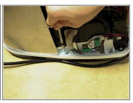
Remove the 4 screws holding the Ice Tray to the body of the Ice Maker.
