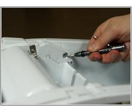
Remove the 4 screws holding the Ice Tray from the top.
