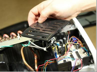
Remove the plastic covering over the circuit board by pressing against the latch on one side. A
