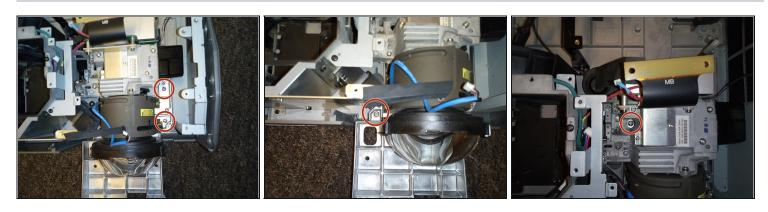
• Remove these 4 silver 9mm Philips #2 screws holding down the main optical system.
