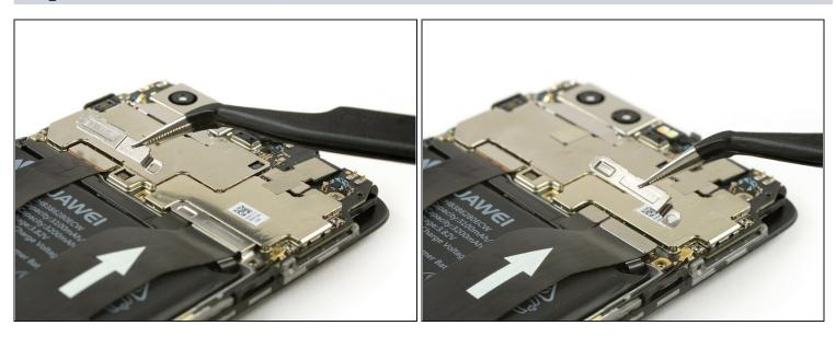
• Use <u>tweezers</u> to remove the two cable brackets.
