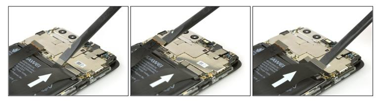
• Use a spudger to disconnect the battery, the interconnect and the display flex cable.
