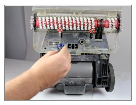
Use a long #2 Philips head screwdriver to remove the 8 numbered screws on the bottom of the cleaner.
