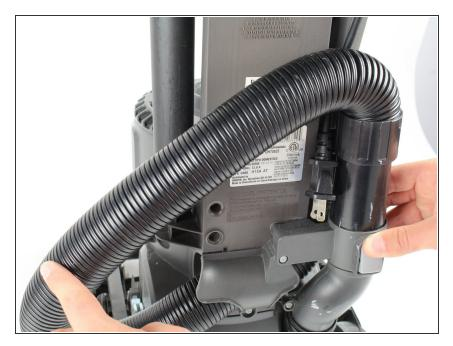
Detach the top of the hose from the device by pressing the release button and pulling up on the hose.
