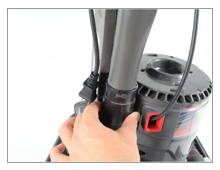
Remove the other end of the hose by twisting the hose clockwise and pulling it off.
