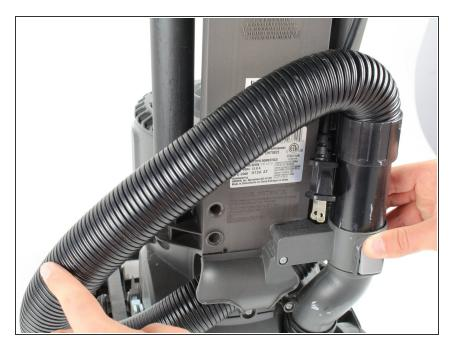
Firmly insert the larger end of the replacement hose into the upward facing hole in the vacuum.
