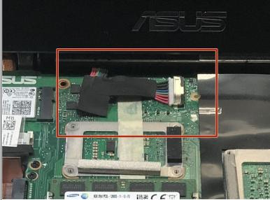
Use a pair of tweezers to carefully disconnect the pin connector.
