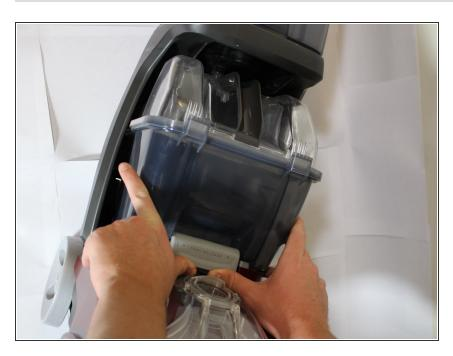
Unlatch the grey switch labeled "Tank Release".
