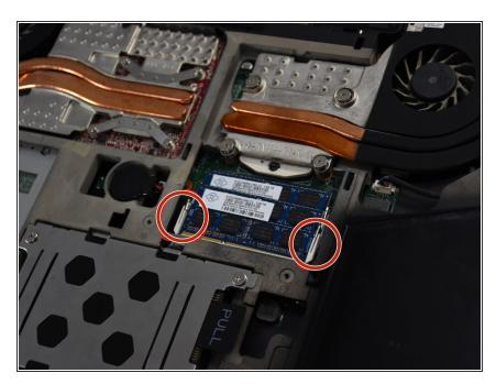
Push the two retaining clips on either side of the ram outwards, allowing the RAM chip to pop up.
