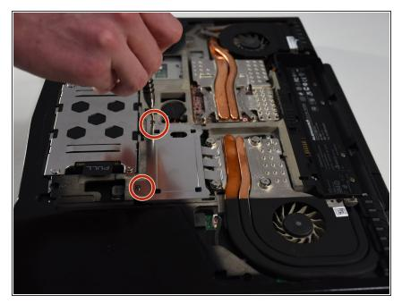
Remove the two indicated screws for the RAM cover.
