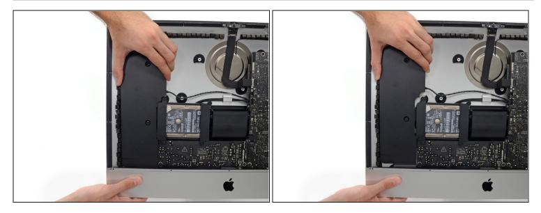
• Lift the left speaker straight up, until the power button cable is exposed (about 0.5").
