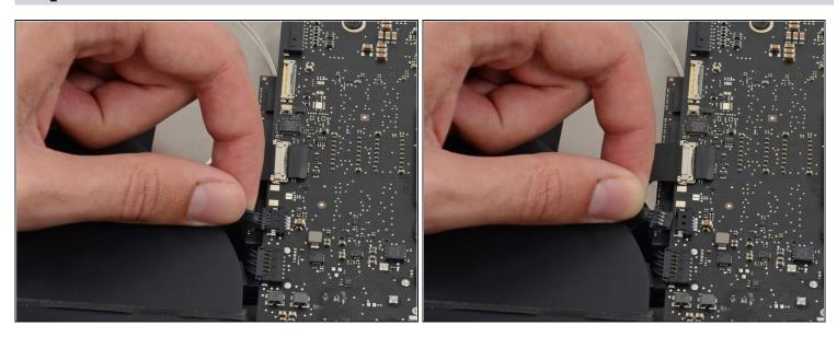
• Gently pull the fan cable connector straight away from its socket on the logic board.
