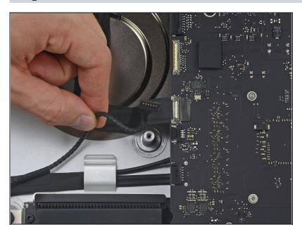
• De-route the left speaker cable by pulling it straight up out of the retaining clip in the back of the rear enclosure.
