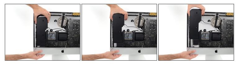
• Lift the left speaker straight up and remove it from the iMac.
