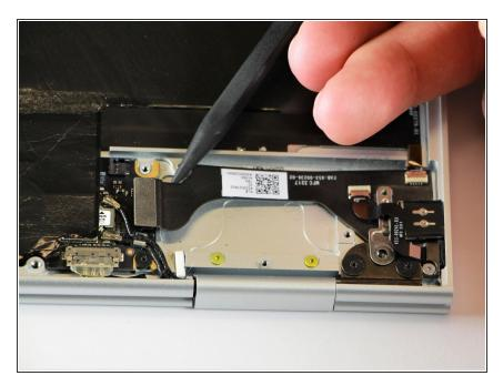
• Disconnect the metal component of the thin, black component by lifting it up with the spudger.
