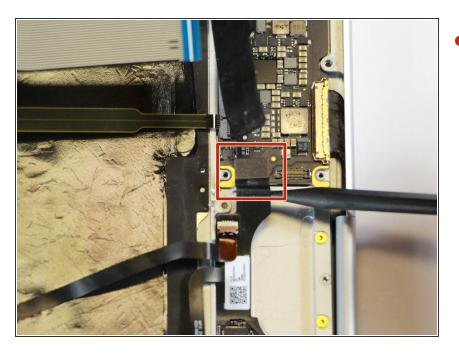
Use the spudger to disconnect the sound card from the motherboard by pulling the connector up and away from the motherboard.
