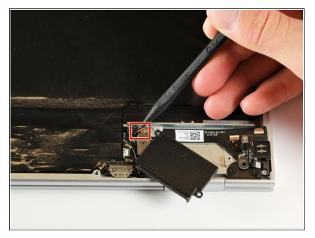
Disconect the thin, black and red cord from the motherboard by using the spudger to snap the connector up and out of place.
