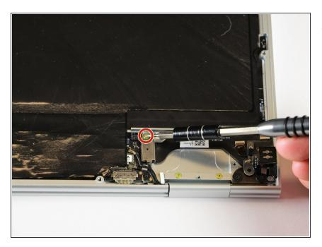
Remove the yellow 2.0mm screw by using the T3 Torx screwdriver to turn the screw counterclockwise.
