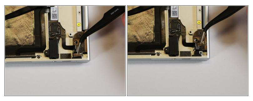
• Use the needle-nose tweezers to remove the silver casing by lifting it up and out of the laptop.
