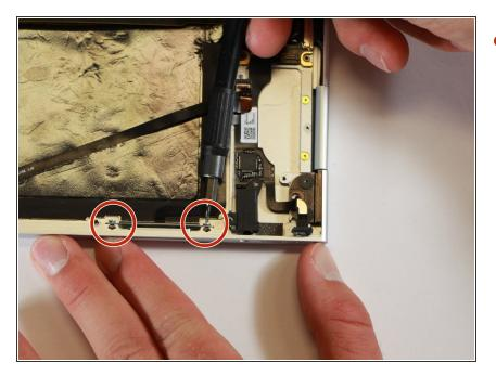
Use a T3 Torx screwdriver to remove the two silver 3.0mm screws located on the vertical edge of the casing by turning the screws counterclockwise.
