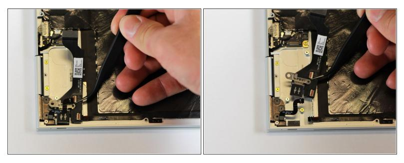
• Remove the right charging port by picking it up with the tweezers and lifting it from the computer.
