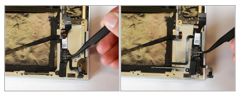
• Use the needle-nose tweezers to remove the sound card by lifting it up and out of the laptop.
