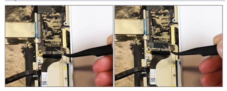
• Using needle-nose <u>tweezers</u>, remove the silver casing by lifting it up and out of the computer.
