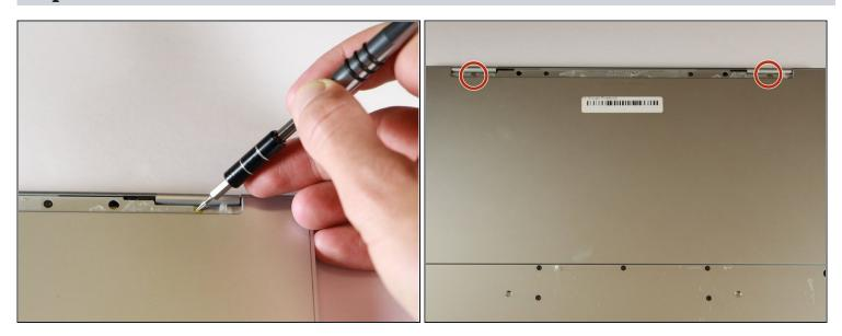
• Remove the two yellow 2.0mm screws by using a T3 Torx screwdriver.
