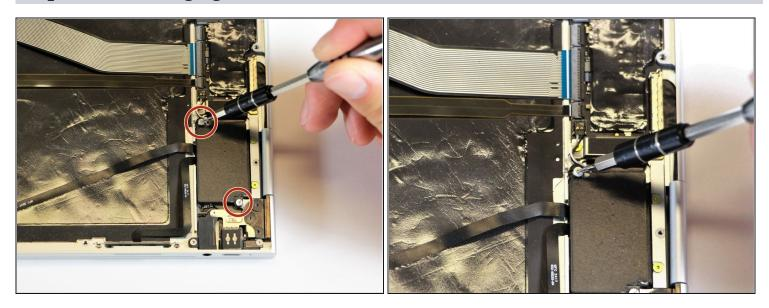
• Remove the two 3.0mm silver screws from the thin, black component by using a T3 Torx screwdriver to turn the screws counterclockwise.
