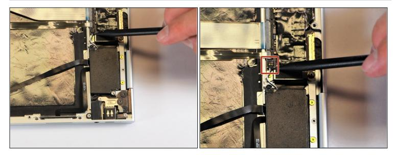
• Disconnect the thin, black and white cord from the motherboard by using the spudger to snap the connector up and out of place.
