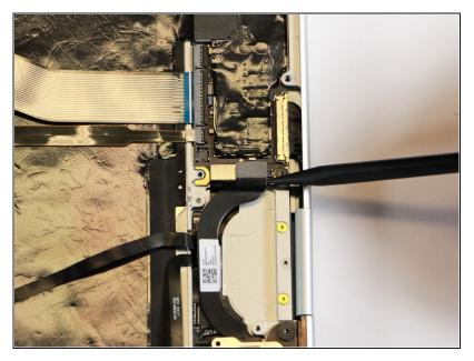
Disconnect the thin, black ribbon cable by using the spudger to lift it up from the computer.
