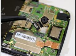
• Disconnect the marked connector with a pair of <u>tweezers</u> and remove the camera piece.
