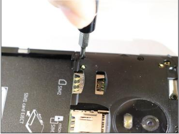
• Remove the eight (8) 4mm screws with a Phillips screwdriver.
